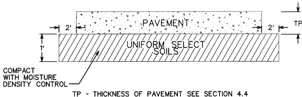
**4.2 SUBGRADE DESIGN (Continued)****FIGURE 4.2 - SUBGRADE WITHOUT UNIFORM SELECT SOILS**
