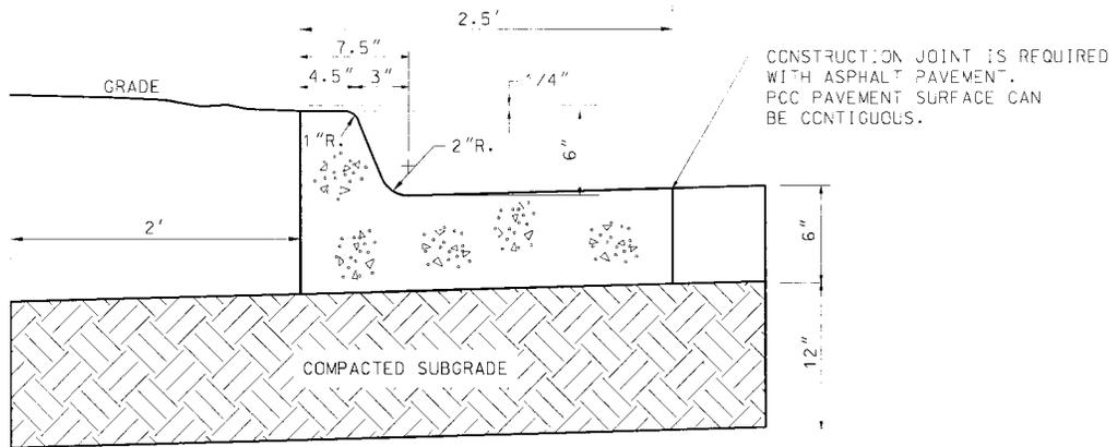
Figure 4.2: Concrete curb and sidewalk combination should be used when storm water flow is desired to flow away from curb.
