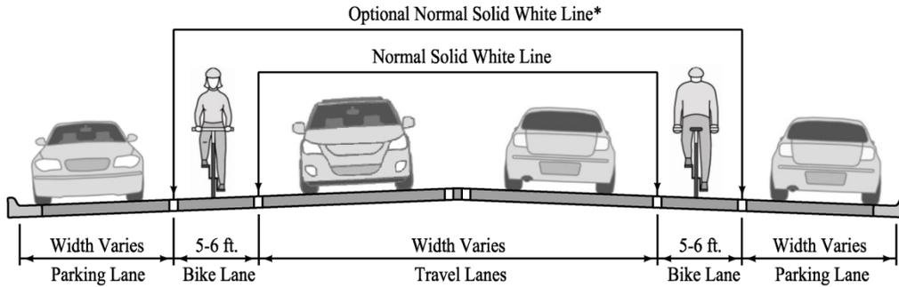
\* The optional normal (4 to 6 inch) solid white line may be helpful even when no stalls are marked (because parking is light), to make the presence of a bicycle lane more evident. Parking stall markings may also be used.
