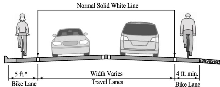
\* On extremely constrained, low-speed roadways with curbs but no gutter, where the preferred bicycle lane width cannot be achieved despite narrowing all other travel lanes to their minimum widths, a 4 foot wide bicycle lane can be used.
