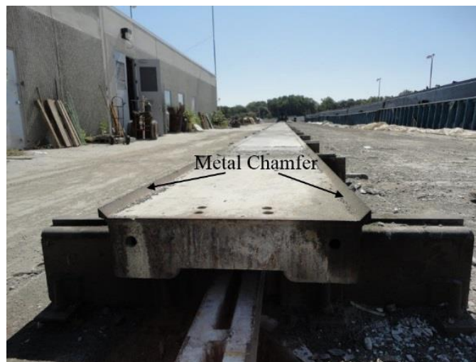
Figure 4.2. Precasting bed with metal chamfer
