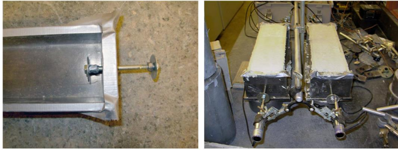
Figure 2.11. Bolt/washer assembly and test setup with LVDTs (Mokarem et al. 2008)
