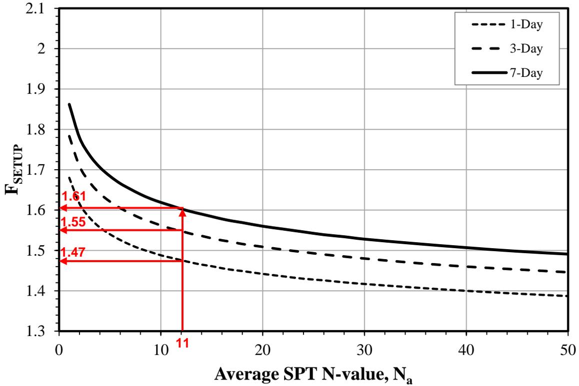
**Figure 5.4. Track 3 Example 1: Pile setup factor chart**
