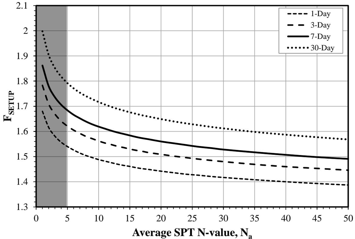
**Figure D.1. Pile setup factor chart for WEAP as a construction control method**
