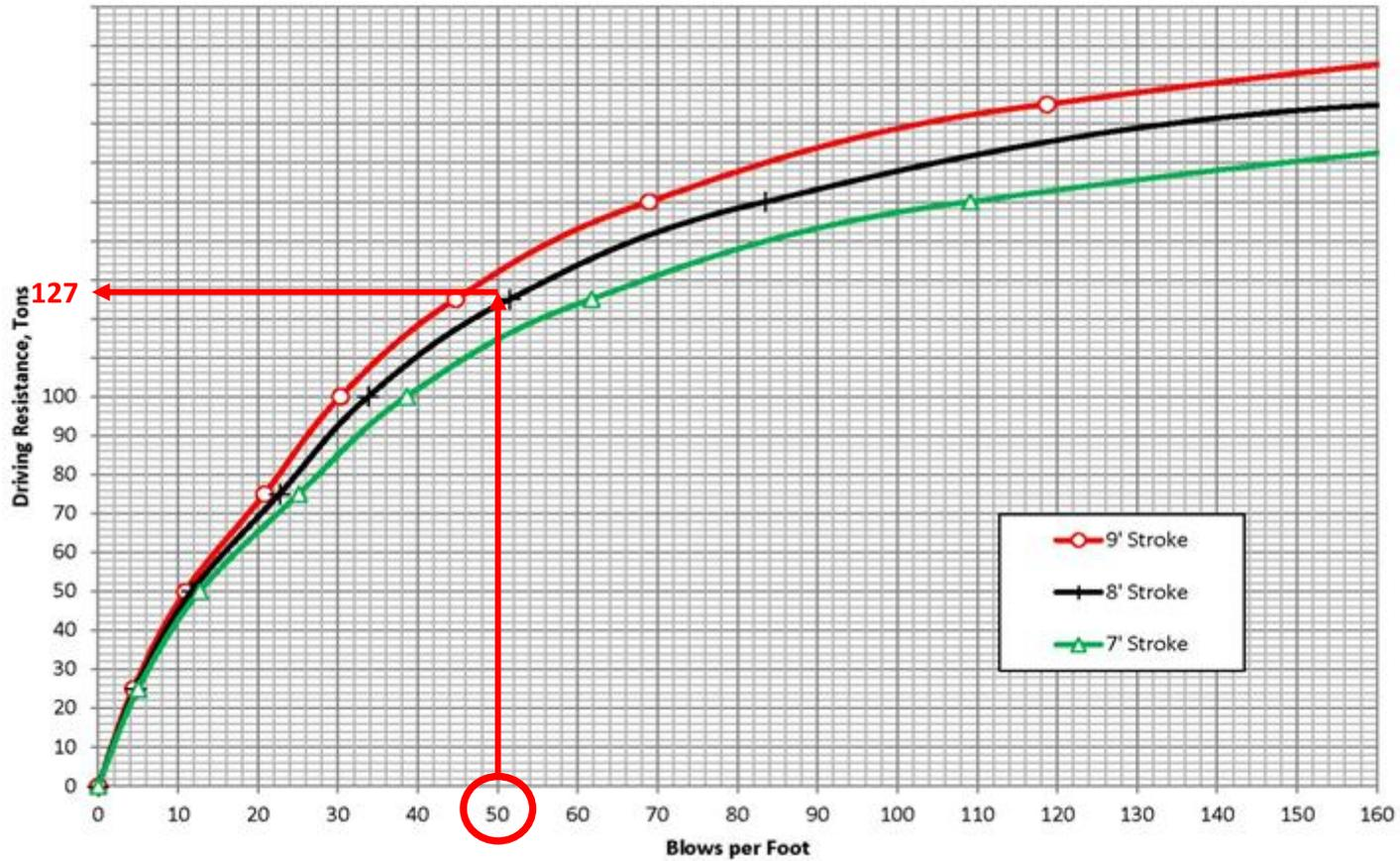
Figure 3.6. Track 1 Example 1: WEAP bearing graph for west abutment piles
