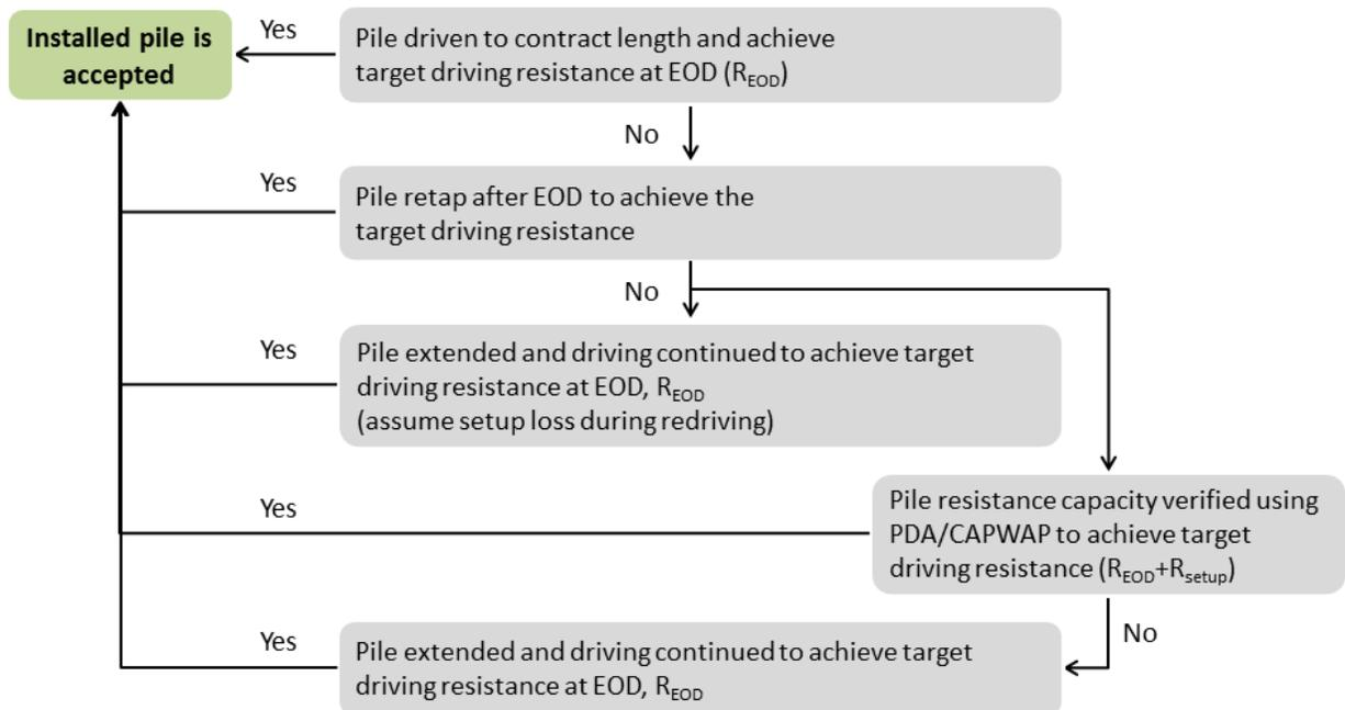
**Figure 2.2. Construction control flow chart for friction piles embedded in cohesive soil and retap performed after EOD**
