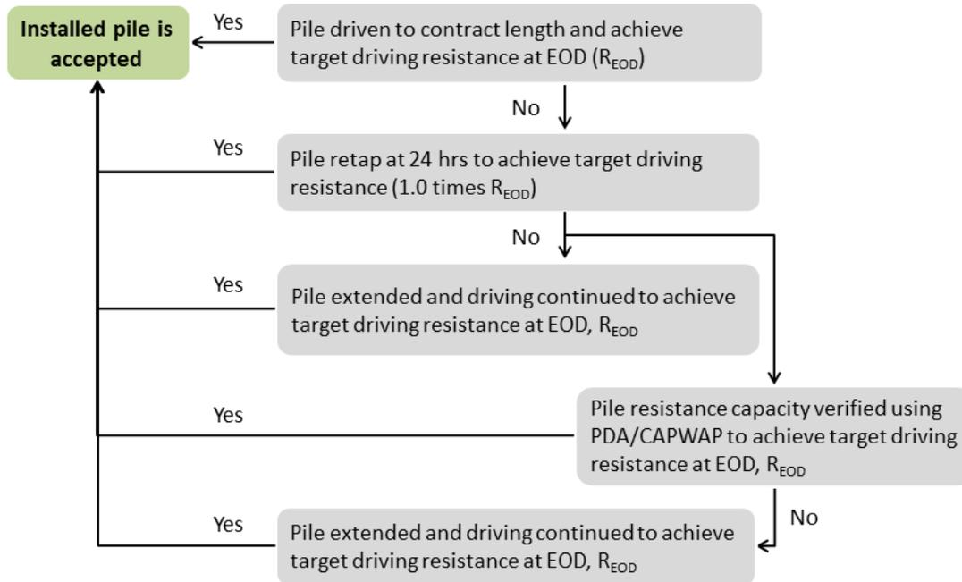
**Figure 2.1. Construction control flow chart for end bearing piles in all soil types and friction piles embedded in non-cohesive and mixed soil types**
