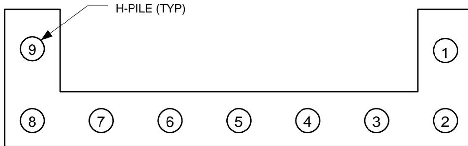
**Figure 5.2. Track 3 Example 1: Pile arrangement at an abutment**
