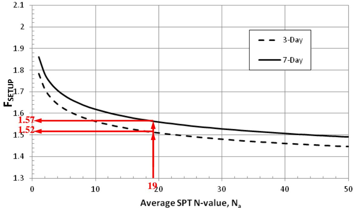
**Figure 5.6. Track 3 Example 2: Pile setup factor chart**
