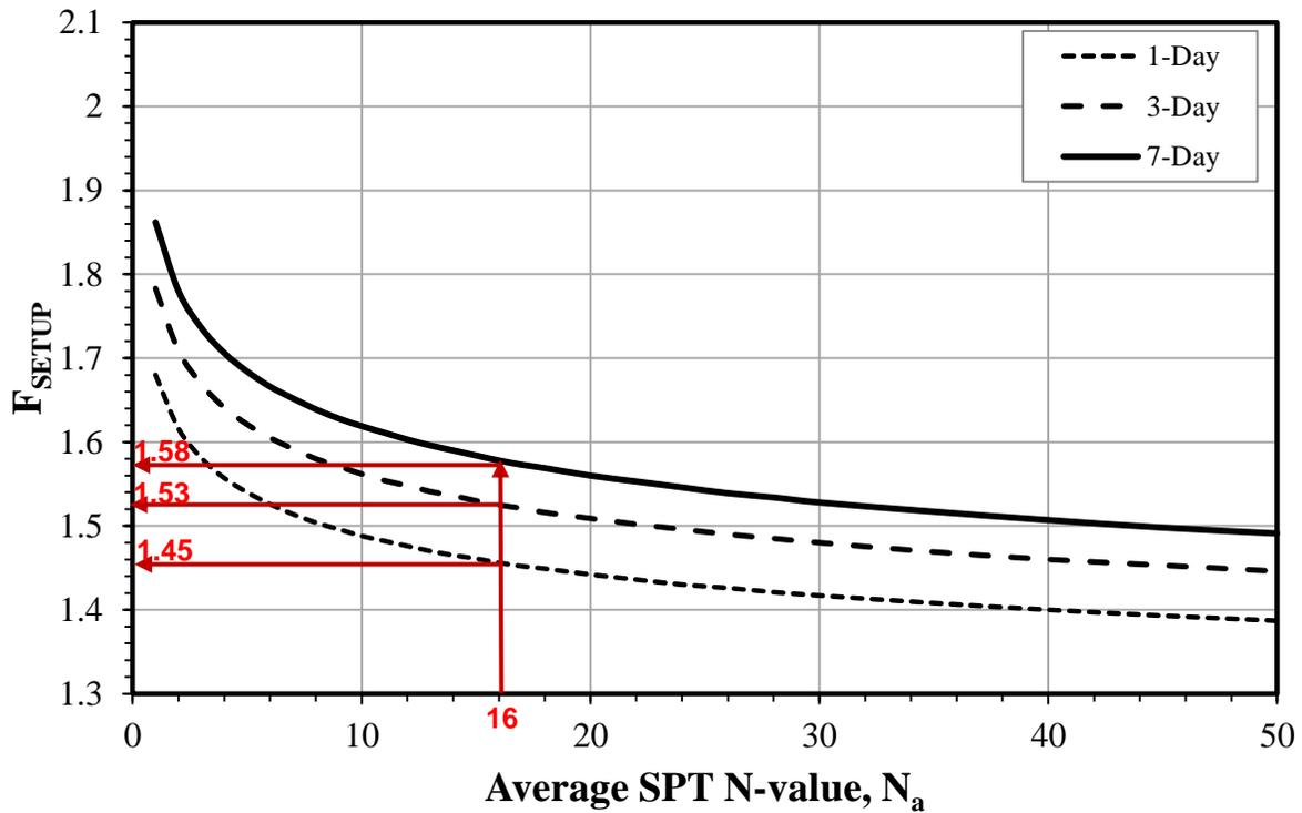
**Figure 3.12. Track 1 Example 3: Pile setup factor chart**
