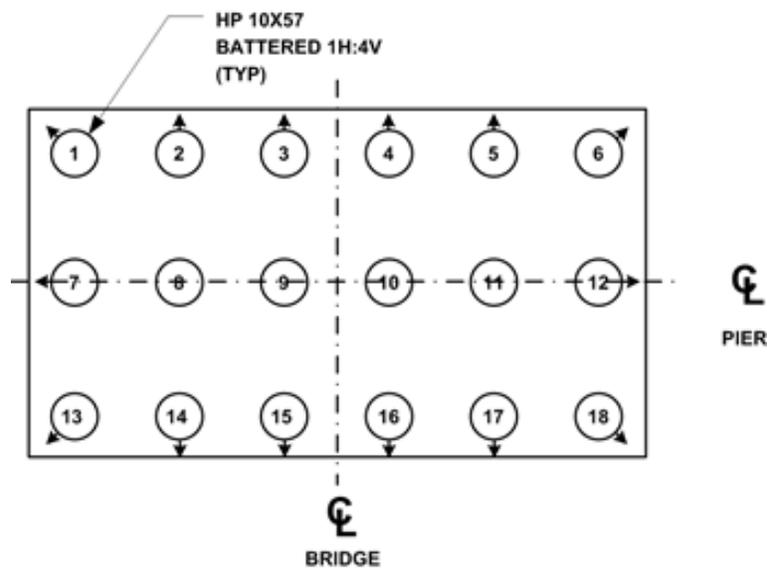
**Figure 3.9. Track 1 Example 2: Pile arrangement at a pier**
