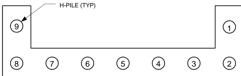
**Figure 4.2. Track 2 Example 1: Pile arrangement at an abutment**
