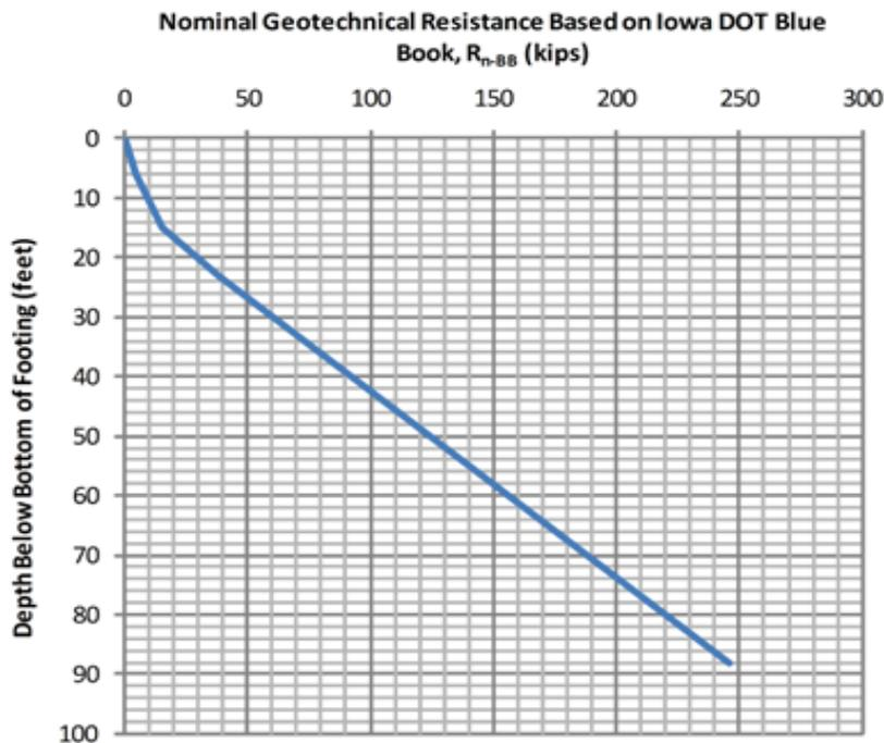
**Figure 3.3. Track 1 Example 1: Plot of nominal geotechnical resistance versus depth**
