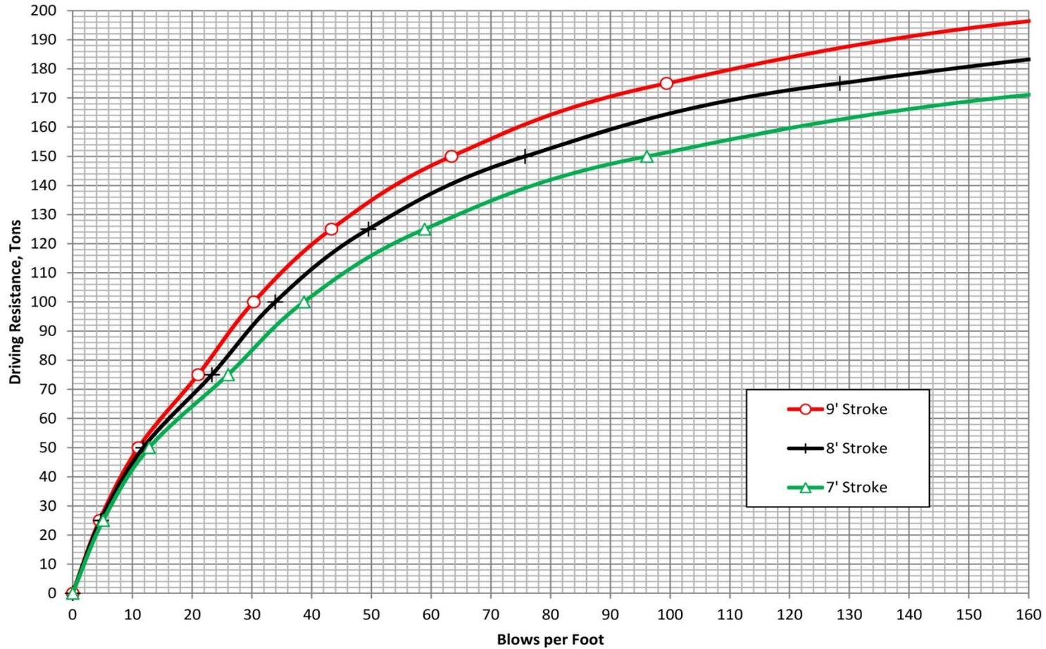
Figure 5.7. Track 3 Example 2: WEAP bearing graph for the west abutment
