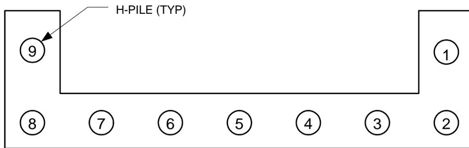
**Figure 5.5. Track 3 Example 2: Pile arrangement at an abutment**
