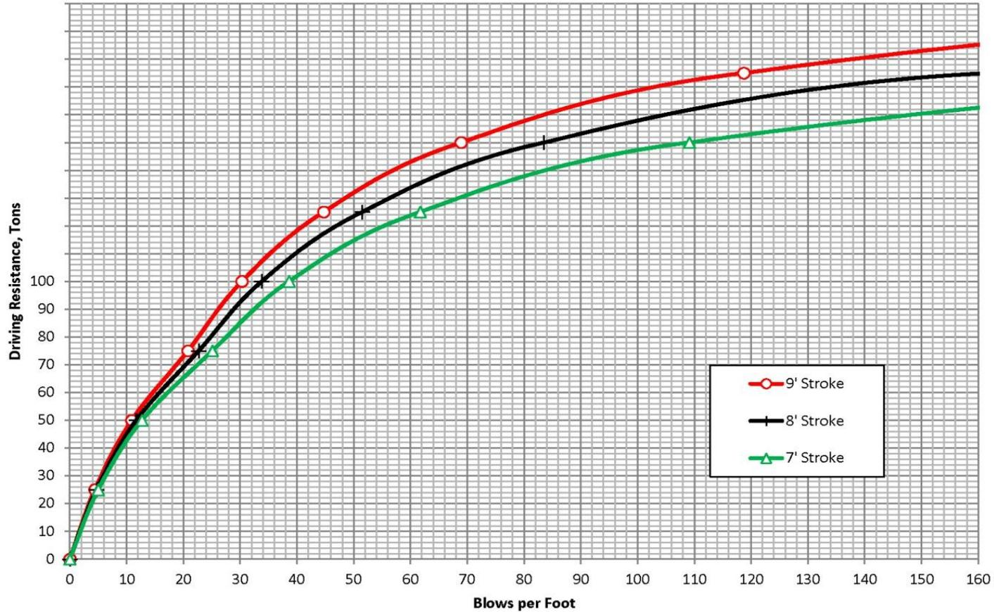
Figure 3.5. Track 1 Example 1: General WEAP bearing graph
