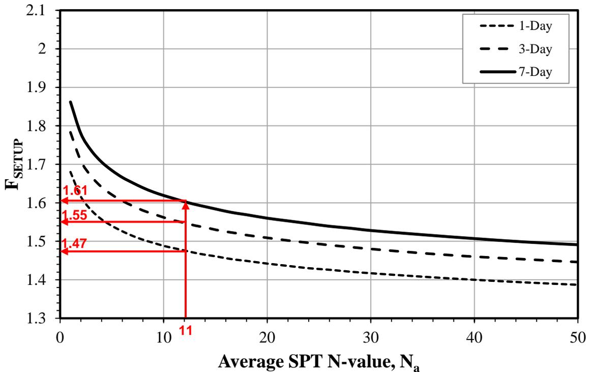
Figure 3.4. Track 1 Example 1: Pile setup factor chart
