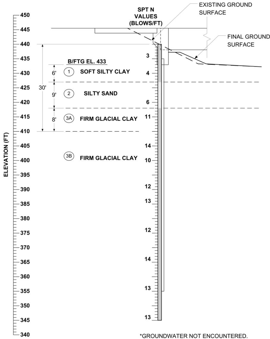
**Figure 5.1. Track 3 Example 1: Soil profile**
