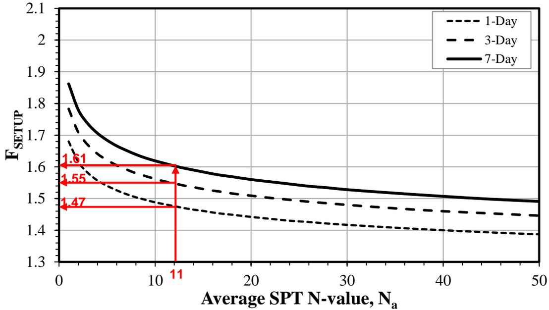
**Figure 4.3. Track 2 Example 1: Pile setup factor chart**
