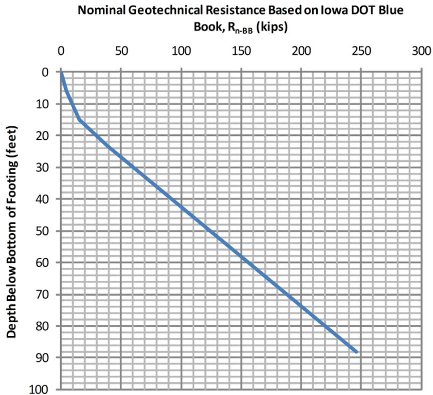
**Figure 5.3. Track 3 Example 1: A plot of nominal geotechnical resistance versus depth**
