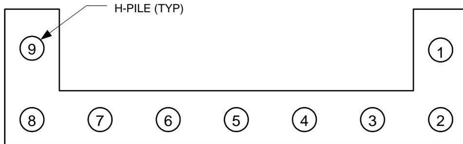
**Figure 3.15. Track 1 Example 5: Pile arrangement at an abutment**
