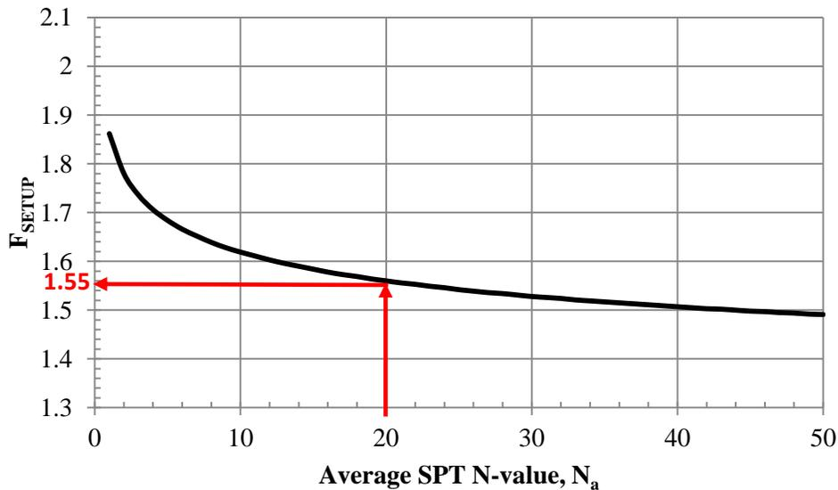
**Figure 3.16. Track 1 Example 5: Pile setup factor chart**
