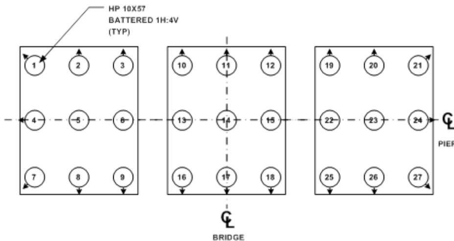
**Figure 3.14. Track 1 Example 4: Pile arrangement at pile piers**
