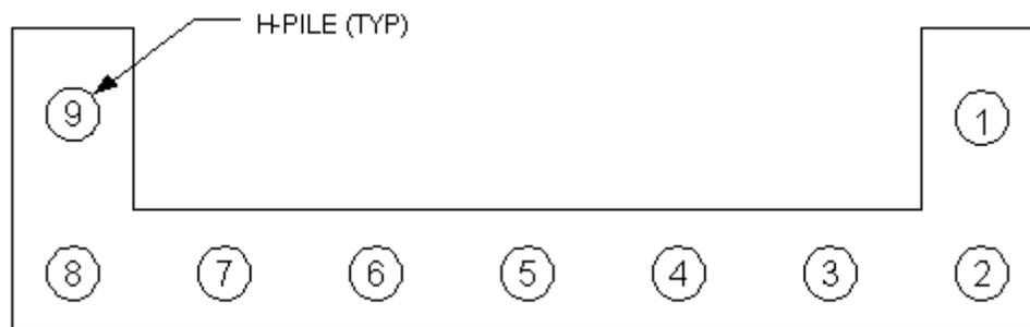
**Figure 3.2. Track 1 Example 1: Pile arrangement at an abutment**
