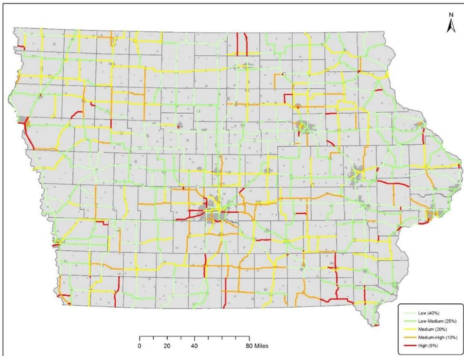
**Figure 44. Route-level primary-road heavy-truck VSIS contact history by density or contacts per mile (top) and by rate or contacts per 100M VMT (bottom)**
