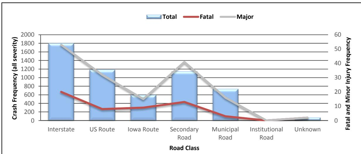
**Figure 22. Single-vehicle crash frequency by road classification 2007 through 2012**
