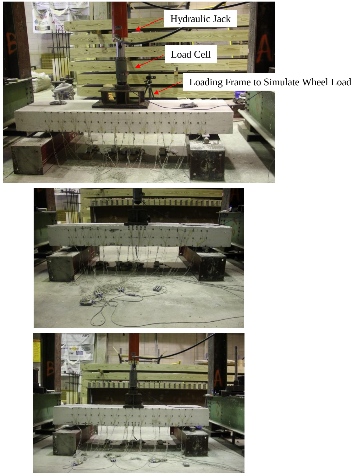
Figure 4.3. Test setup for Specimens NO (top), OT (center), and OB (bottom)
