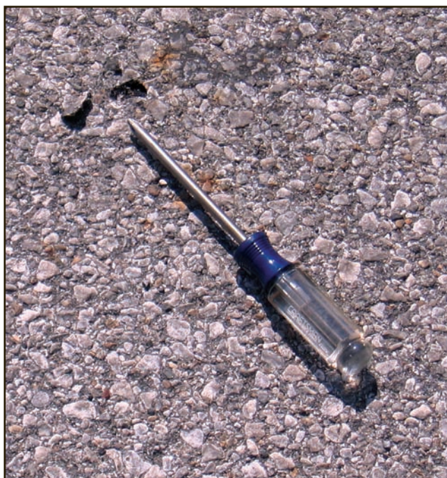
Figure 2. Use of a screwdriver to dislodge aggregate can help test the degree of oxidation on the pavement.
