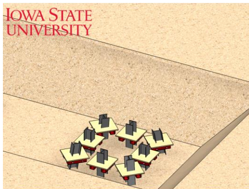
3. Plywood sealing the pile sockets
