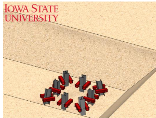
2. Friction collars shoring precast pile cap
