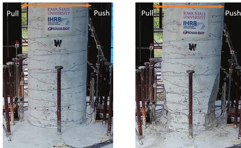
Figure 5.41. Damage at the column base: flexural cracks (left) and cover concrete spalling (right)
