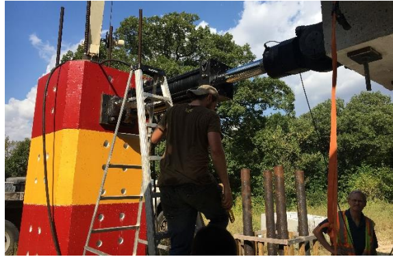
Figure 5.28. Lateral actuator attached on reaction column
