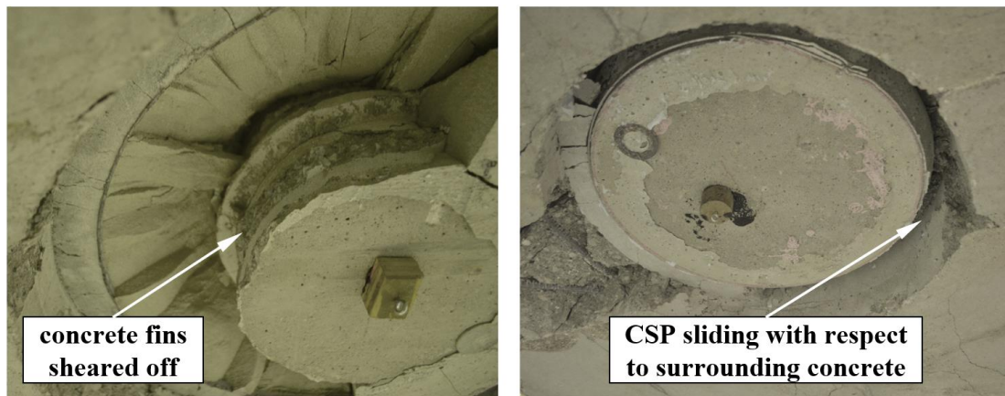
Figure 4.10. Failure modes of the specimens
