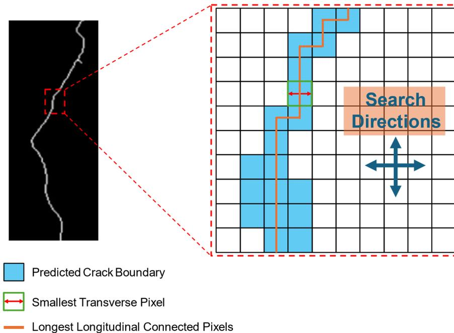
**Figure 4.4. Illustration of region-growing algorithm**
