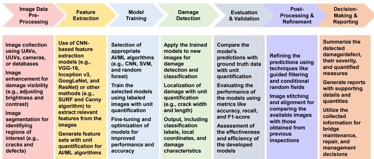
**Figure 2.6. Recommended steps for bridge maintenance and management based on the instances of damage/defects detected using AI/ML techniques**
