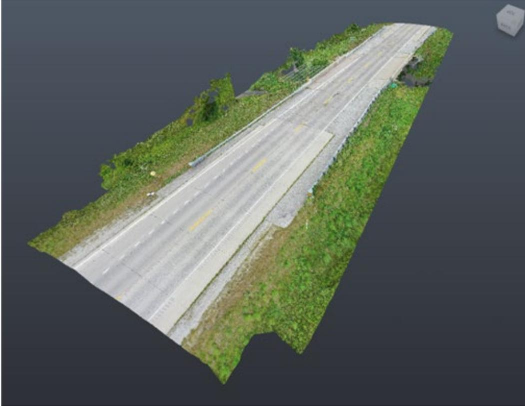
**Figure 3.12. 3D model generated by Autodesk ReCap Pro**
