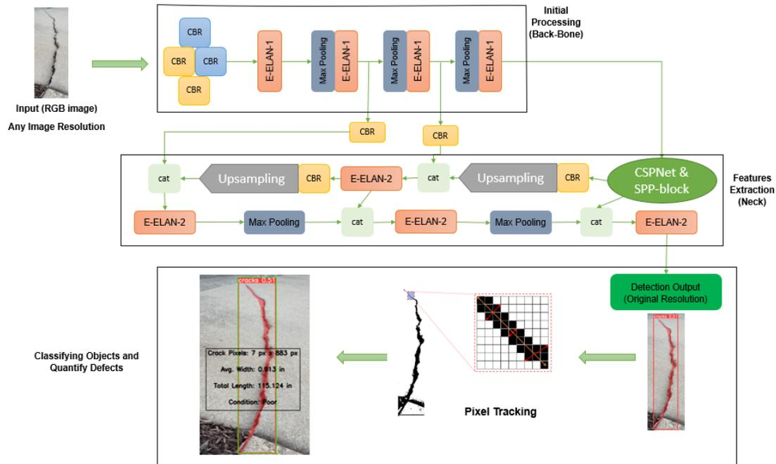
**Figure 4.6. New proposed quantification and assessment model**
