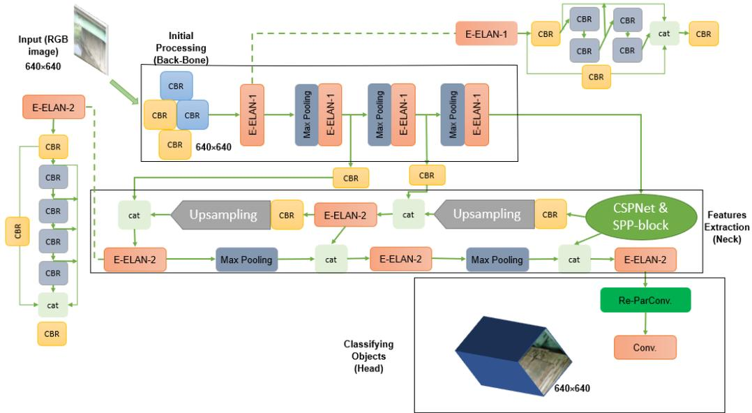
**Figure 4.3. Original YOLOv7 network structure**
