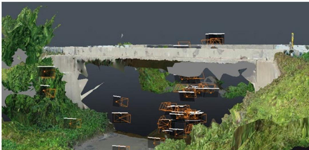
**Figure 3.16. Image locations and positions not used to generate the 3D model**
