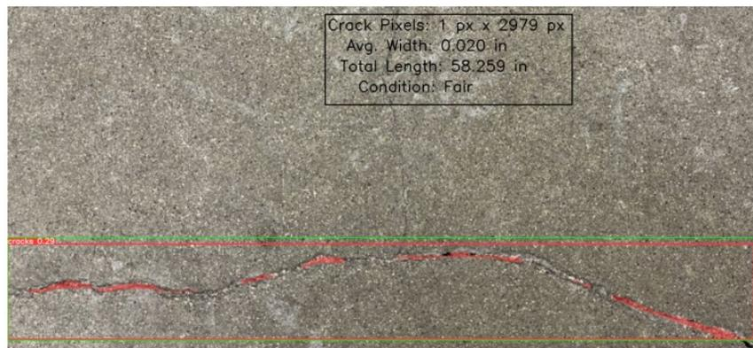
**Figure 4.23. Result of crack quantification with different assessment**
