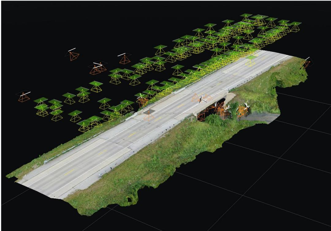
**Figure 3.15. Image locations and positions used to generate the 3D model**
