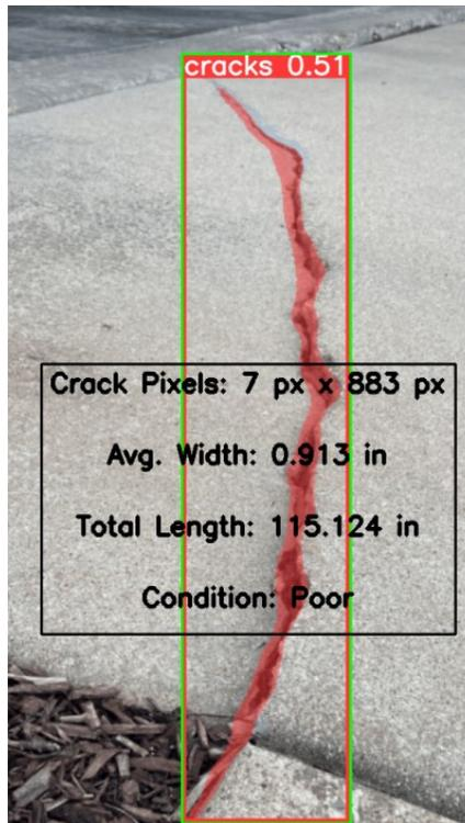
**Figure 4.22. Result of crack quantification**
