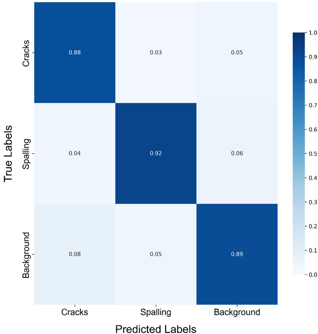
**Figure 4.12. Confusion matrix of the developed model**
