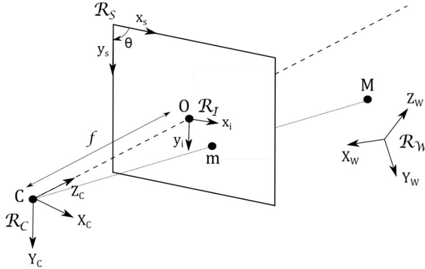
**Figure 4.5. Illustration of camera calibration**
