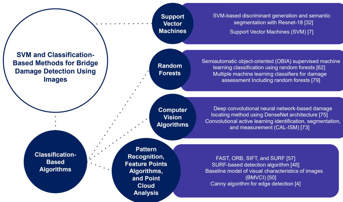
**Figure 2.5. Overview of SVM and classification-based algorithms used to detect bridge damage**
