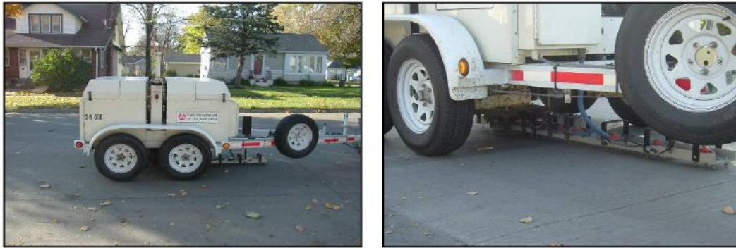
Figure 9D-1.06: Iowa DOT FWD Equipment Showing Sensor Configuration
