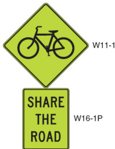
Figure 12B-3.01: Share the Road Sign Assembly
