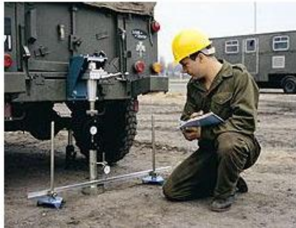
Figure 6E-1.01: In-situ CBR
